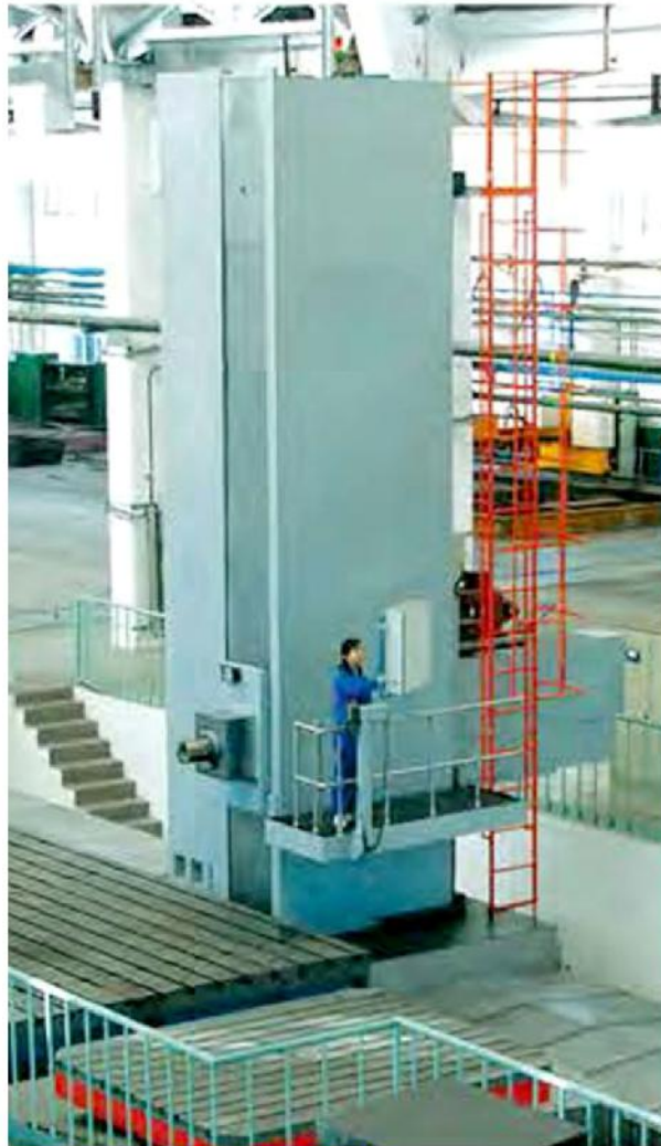
TH69(13/16/20/26)B CNC Floor boring-milling machine
