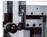
机内对刀装置 Internal Device for Cutting Tool Pre-Setting
